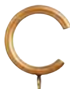
CR-SR12 smooth steel c-ring 2 5/8"ID, 3"OD use with RR175 or RD175 pole and SCB35, SCB6, SCBC or SCBCDBL bypass brackets
